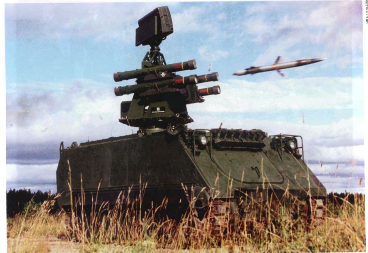
The ASRAD-R on the M113 chassis. The system can be installed on a range of tracked or wheeled carrier vehicles.
